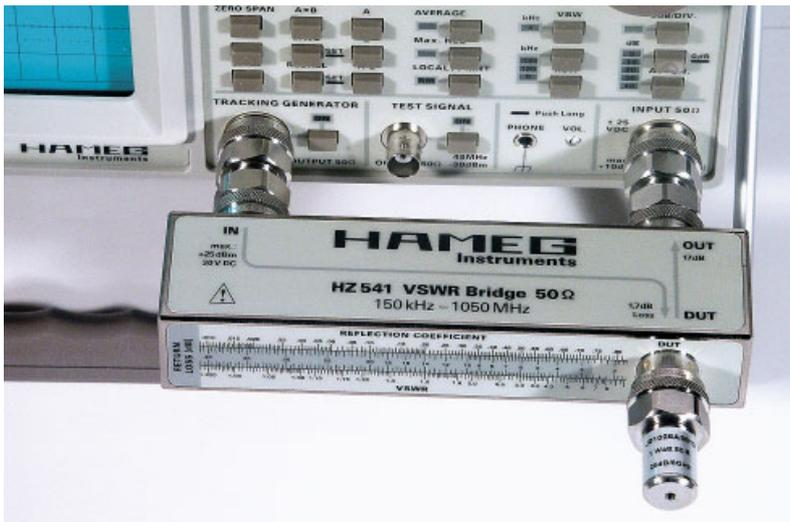
Connect the IN input to the tracking generator of the HM 5014-2 (signal source)
