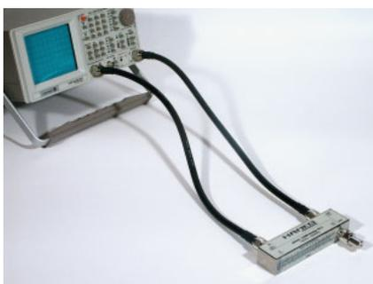
In case a spectrum analyzer of another manufacturer is used the adapters have to be replaced by N cables (optional).
